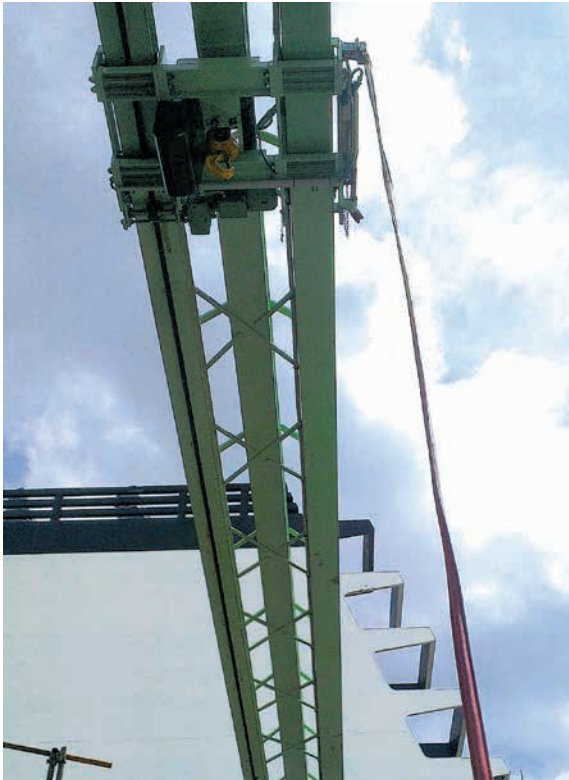
Deck Gantry Crane SWL 5.0t Class BV Span 15.5m
