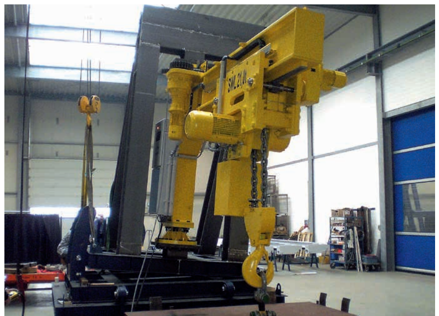
Slewing Jib Crane SWL 21t Outreach 3675 mm Class BV
