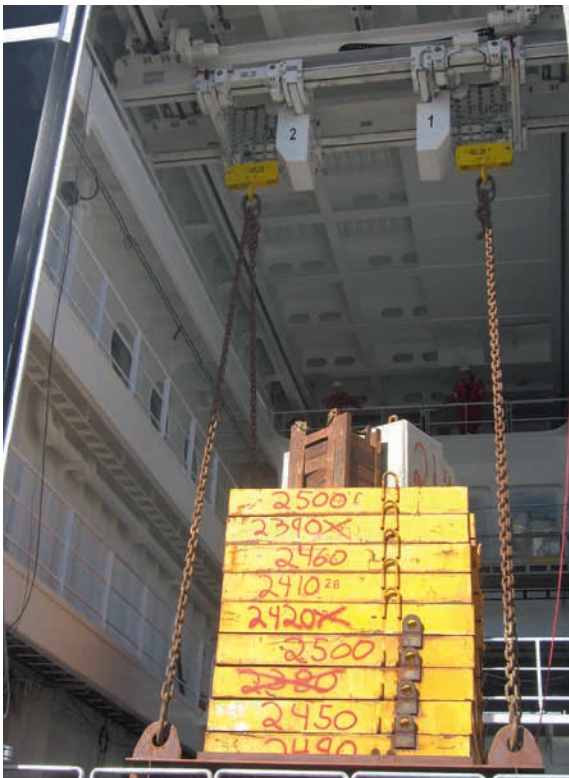
ROV Hangar Crane SWL 2x 25t Class DNV
