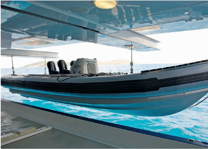
Electric Tender Boat Crane SWL Fwd 2 x 2.5t / Aft 4 x 2.0t Outreach 3950mm over both ship sides Class LR
